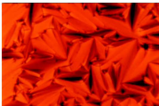
Fig. 1. Fan-shaped texture of smectic A of 4a , crossed polarizers, 100 × magnification, 57.5 °C.
